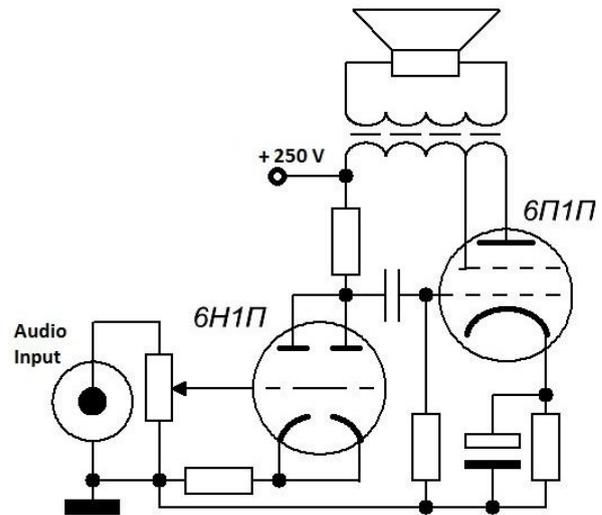
Fig. 2. Circuit of tube amplifier device
