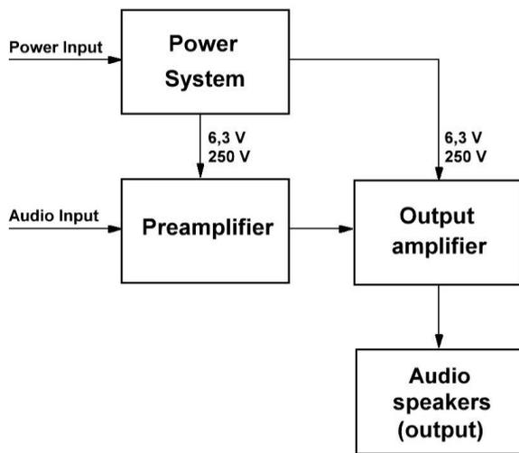
Fig. 1. Block scheme of tube amplifier
