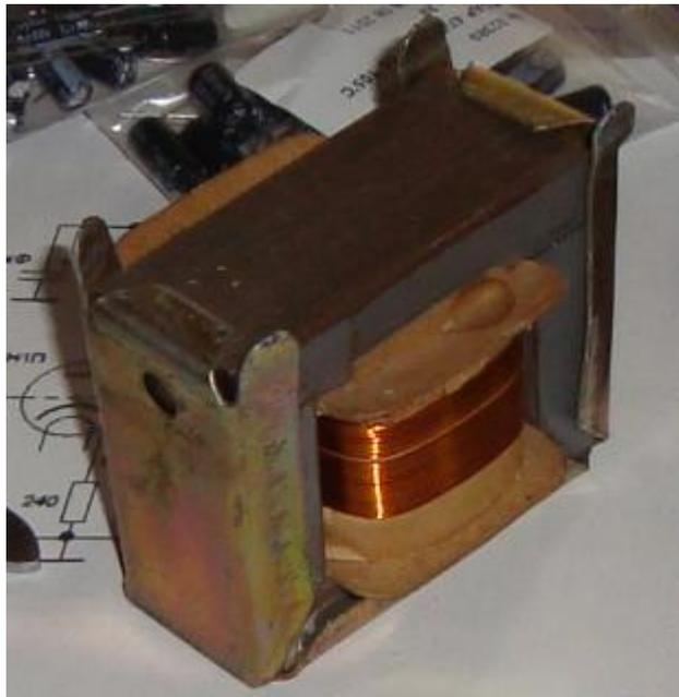
**Fig. 4. Output audio transformer**
