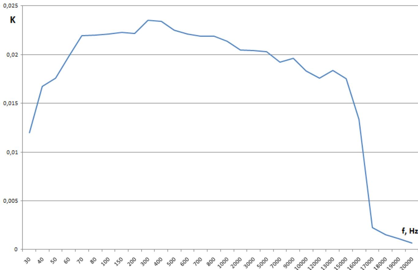
**Fig. 5. Amplitude-frequency characteristics of audio output transformer**
