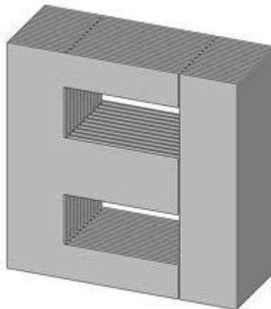
**Fig. 3. EI type of transformer core**
