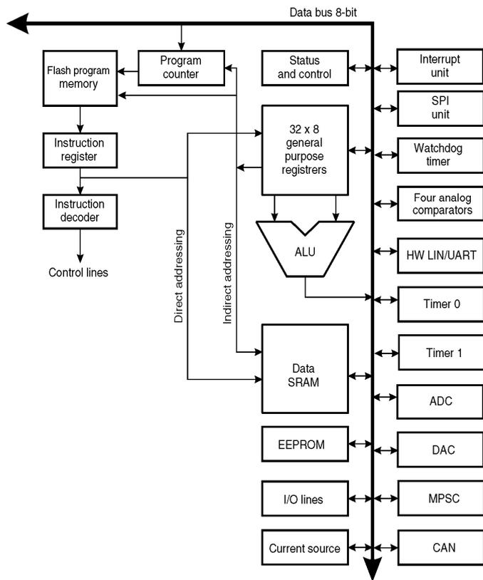
Fig. 8. The structure of the microcontroller ATmega16M1 [9]
