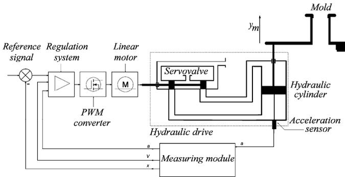
Fig. 4. The structure of mold oscillation system
