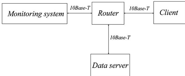
Fig. 11. The structure of the control network of the factory
