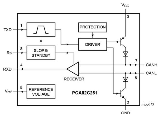
Fig. 10. The structure of the chip PCA82C251 [10]
