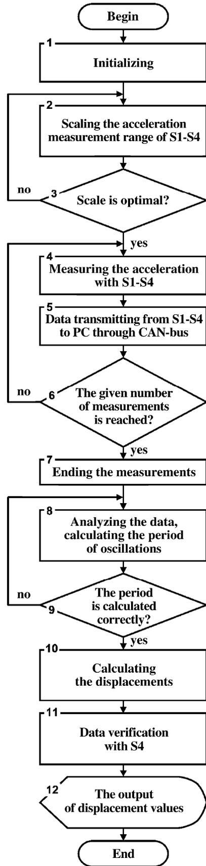
Fig. 7. The algorithm of the measurement system operation
