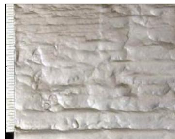
Fig. 3. The defects of slab billet [3].
