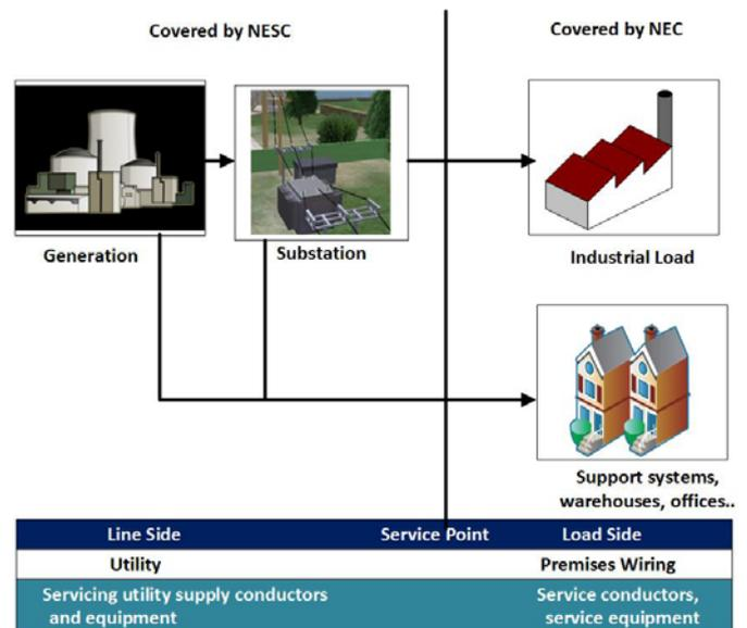
Figure 2 Scope of NESC and NEC [9, 12]
