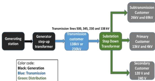
Figure 1 Basic electric system structure [11]
