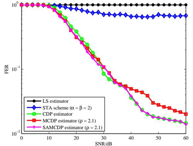
Fig. 6. Comparison of the FER performance of LS, STA, CDP, MCDP, and SAMCDP in QPSK modulation (V2V Expressway Oncoming).
