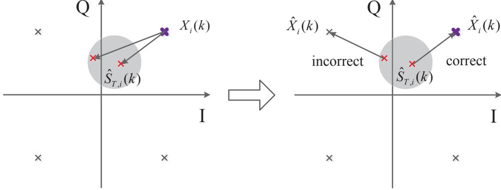
Fig. 3. Schematic diagram of constructing data pilot.
