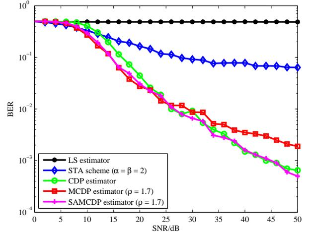
Fig. 5. Comparison of the BER performance of LS, STA, CDP, MCDP, and SAMCDP in QPSK modulation (R2V Suburban Street).
