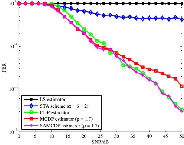
Fig. 7. Comparison of the FER performance of LS, STA, CDP, MCDP, and SAMCDP in QPSK modulation (R2V Suburban Street).
