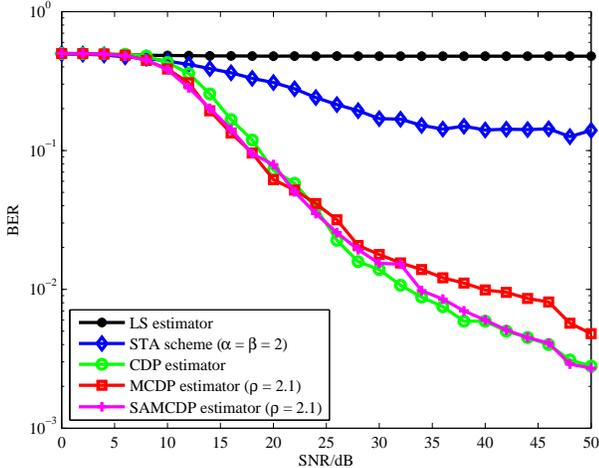
Fig. 4. Comparison of the BER performance of LS, STA, CDP, MCDP, and SAMCDP in QPSK modulation (V2V Expressway Oncoming).
