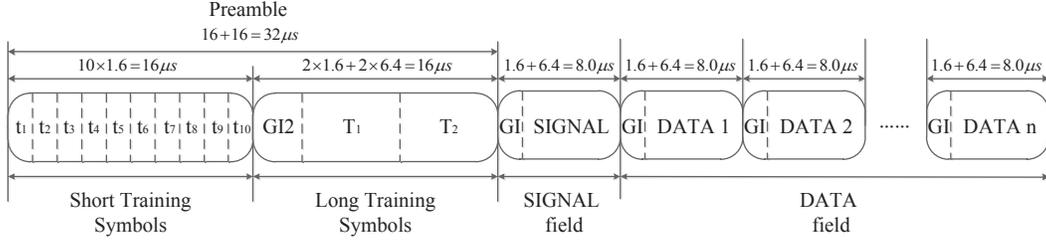
Fig. 1. IEEE 802.11p packet preamble structure.
